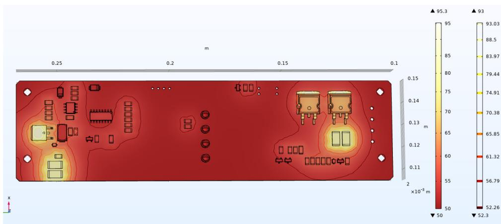
Fig. 5. Thermal gradient simulation result in Comsol Multiphysics.
