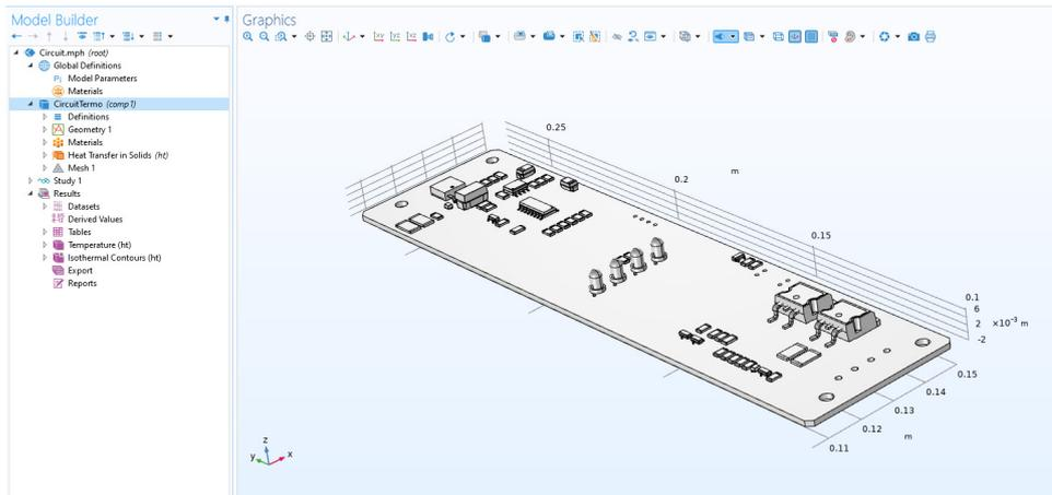
Fig. 4. The result of importing a model into COMSOL Multiphysics from SolidWorks.
